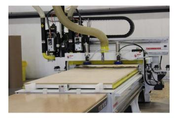
The Framebuilder system is a fixed table machine which makes automatic load and unload extremely simple and straightforward. The operation starts with a scissor lift located at the front of the fixed machine table. A stack of sheet material is placed on this scissor lift and it keeps the top sheet just above the level of the machine table. On the initial cycle when a sheet of material is needed, the gantry moves forward and lifts the top sheet using a series of
