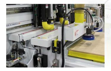
Roller Hold Down is key to machining upholstered frames which present special hold-down problems. The rough surface and tendency to warp make them difficult or impossible to hold with vacuum. In many frame applications, nests are random, so conventional vacuum fixtures cannot be used. The only answer is a roller holddown, a system first developed by Thermwood.
