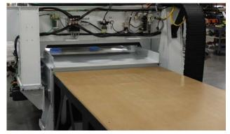
sheet. As the gantry pulls back to load the sheet on the table, the unload bar drops to simultaneously push the machined parts off the back of the table to a sorting table. During this process a built-in dust collection hood on the rake bar cleans the table surface, along with the side table bars automatically raised to keep the parts from sliding off the sides of the table. The machine is now ready to begin the machining process again.
