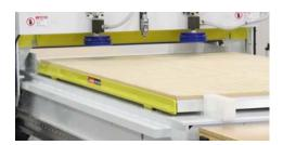
**Programmable Side Bars and Locator Pin** Individually programmable table side bars for providing ease of sheet positioning and unloading. In addition, a programmable, heavy-duty, locator pin is located at the rear of the table work zone for sheet positioning.
